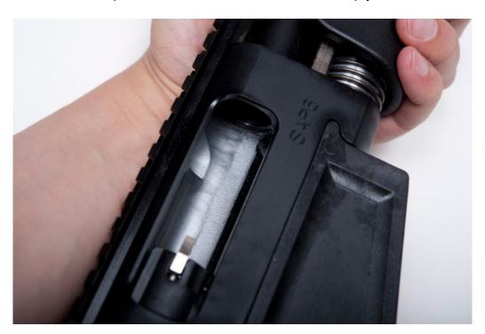
1.4 Remove the collapsible stock by depressing the button on the right side of the stock next to the pistol grip and pull the stock away from the pistol grip.
