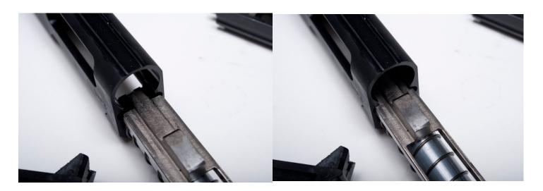
2.2 Insert bolt onto the raised portion of the action bar while sliding the action bar into the receiver.
