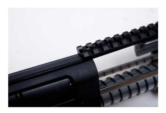
2.6 Once the barrel extension begins to go into the receiver, pull the forend back so the bolt will go rearward to allow the barrel to slide in without obstruction.
