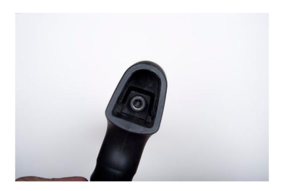
1.15 Once the allen screw is removed, the pistol grip will separate from the receiver.
