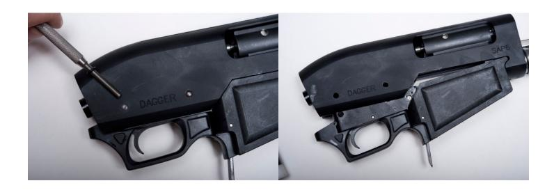
1.17 Be careful when removing the trigger group and magazine-well assembly as the bolt and forend assembly will shoot out and away from the receiver.
