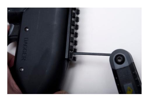
1.9 Two allen screws removed. Keep in mind the one screwed onto the receiver may be longer than the other.
