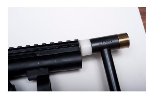
2.8 Photo shown indicates full alignment of the barrel/rail assembly with the receiver with the bolt forward.
