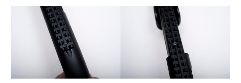
1.8 Remove the two allen screws by using a size 2.5 allen key. Be careful not to misplace them.
