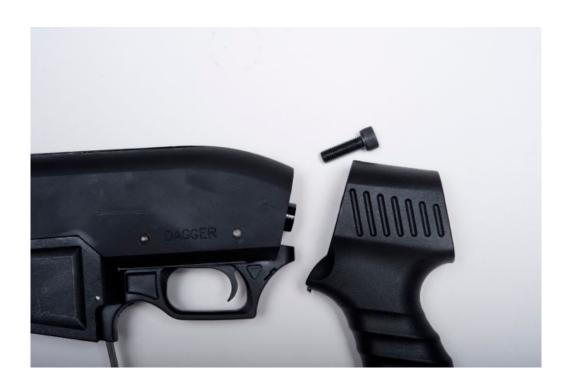
2.12 Insert collapsible stock by depressing the button on the stock and inserting it into the pistol grip assembly at the same time. Assembly is now complete. Be sure to do a quick function test by turning the safety off and racking the forend back and press trigger with gun pointed at safe direction to ensure proper function of firearm.
