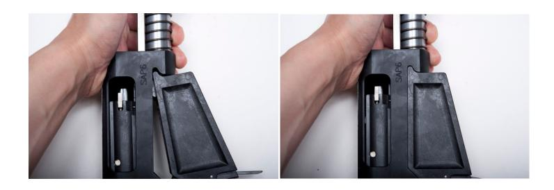
2.4 Tap the two pins back into the receiver with rubber mallet or small hammer with plastic head.
