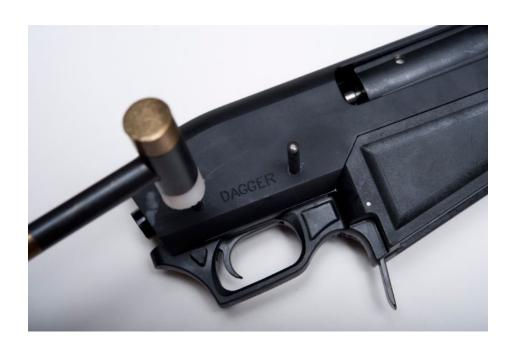
2.5 Slide barrel/rail assembly by first lining up and sliding the monolithic rail onto the receiver dovetail.
