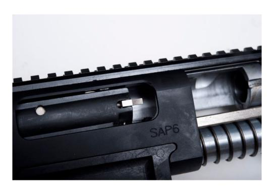
2.7 With the forend still pulled back, slowly and carefully tap the barrel into the receiver.
